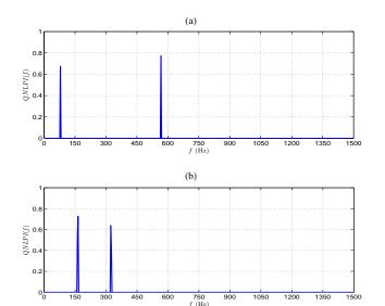
Fig. 6. QNLPI of the AHB: baseline (00321) in (a), and misaligned (20321) in (b)
