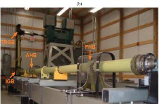
Fig. 3. (a) Actual TRDT on AH-64, and (b) TRDT test stand at USC
