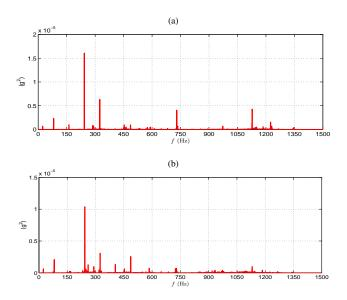
Fig. 5. Power spectral density of the AHB: unbalanced (10321) in (a), and misaligned-unbalanced (30321) in (b)
