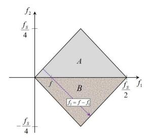
Fig. 1. Region of computation (ROC) for the bispectrum/bicoherence assuming aliasing is absent: triangle "A" is the conventional ROC, region "A-B" is used to calculate the proposed QNLPI(f), and dashed line indicates the direction of integration to calculate the QNLPI(f)
