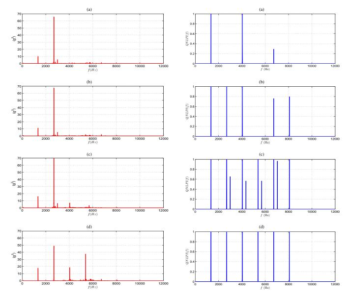
Fig. 9. Progress of power spectral density (PSD) change during gear teeth failure: (a) 3 days before failure, (b) 2 days before failure, (c) 1 days before failure, and (d) same day of failure
