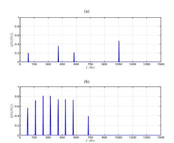
Fig. 7. QNLPI of the AHB: unbalanced (10321) in (a), and misaligned-unbalanced (30321) in (b)
