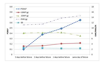
Fig. 11. Trend of vibration PQNLP compared to different condition indicators for the faulted TRGB during the last four days before failure
