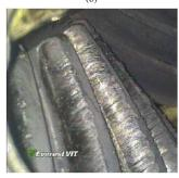
Fig. 8. Borescope picture showing input gear teeth: (a) earlier stage of testing, and (b) after failure [31]
